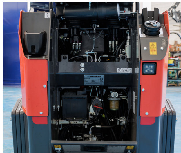
Rear access to battery and pump.
