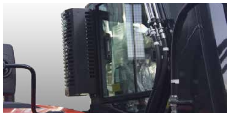
Hydraulic preparation for mulcher with additional pump (max. 57 lt/min, maximum pressure 180 bar) complete with: external air conditioning system condenser and blowing fan.
