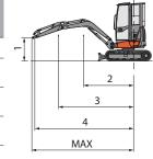
The lifting capacity is based on the ISO 10567 and it does not exceed more than the 75% of static tipping load or more than the 87% of the hydraulic lifting capacity of the machine.
