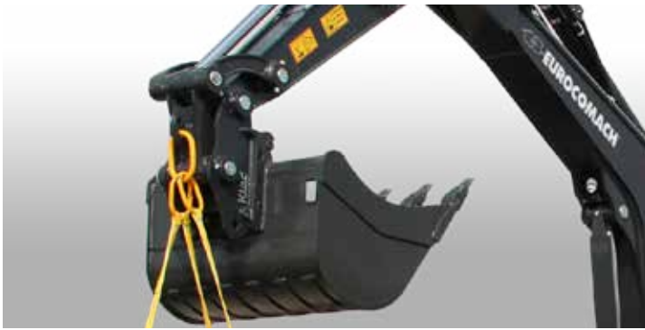
Certified and tested lifting hook with blocking valves with CE certification for material handling equipment
