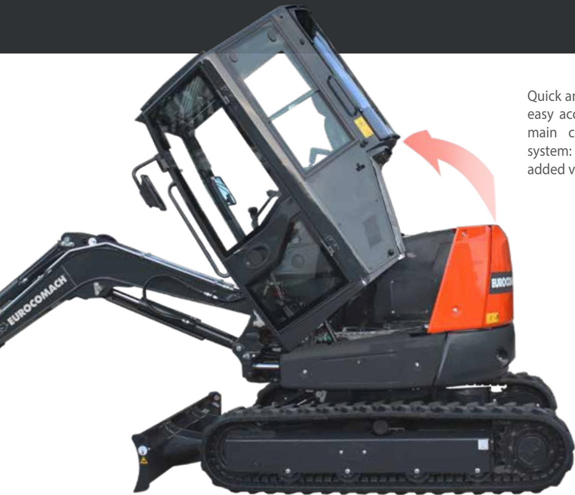
Quick and easy tipping of the cab gives easy access to the distributor and the main components of the hydraulic system: just a few gestures for major added value.
