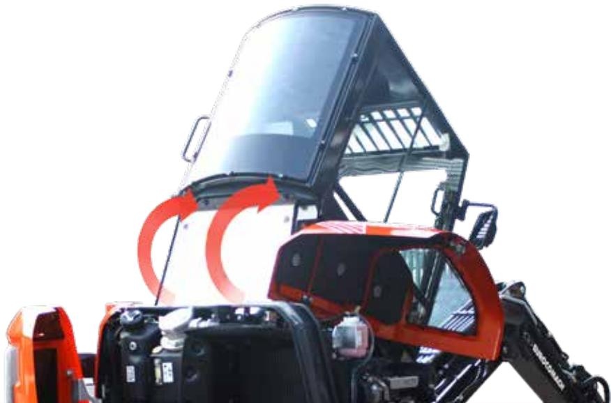
Easy routine maintenance simplifies service operations. The rear bonnet allows quick cleaning of the radiator and access to the oil and fuel tank.
