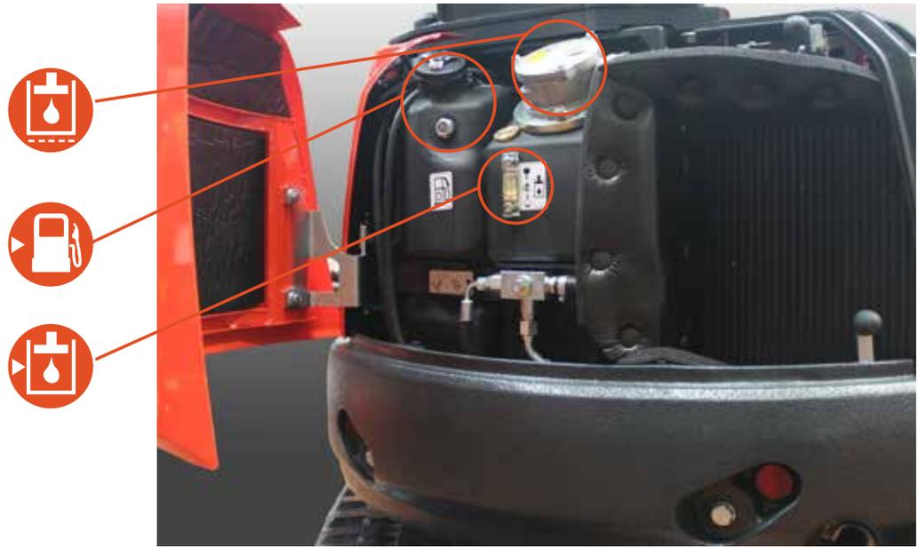
Services related to the heat engine are easily reached through a wide opening and the side compartment. All the filters (fuel, oil and air) in addition to checking and topping up the engine oil, are easily identified on the side.
