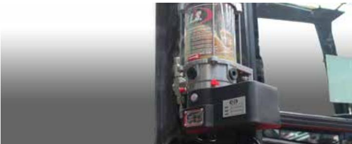
Automatic centralized lubrication
