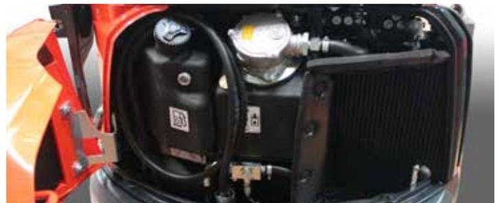
Electronically controlled diesel filler pump
