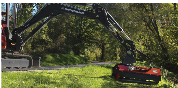
Hydraulic system for chopper with additional pump (22 lt/min)
