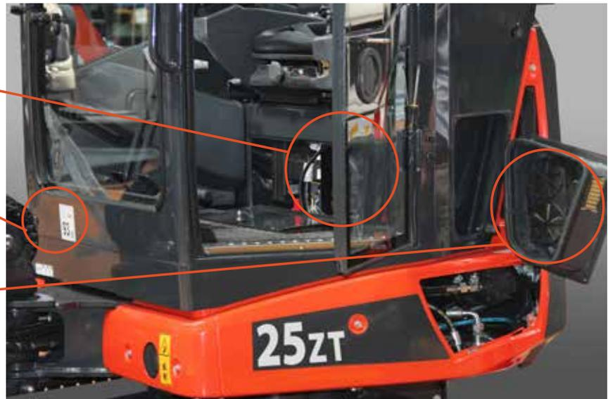
The location of the cabin aeration filters allow them to be quickly checked and replaced if necessary.
