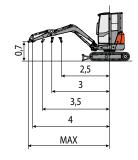
The lifting capacity is based on the ISO 10567 and it does not exceed more than the 75% of static tipping load or more than the 87% of the hydraulic lifting capacity of the machine.
